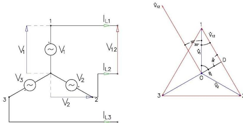
$$\begin{aligned} \dot{V}_{12} &= \dot{V}_1 - \dot{V}_2 \\ \overline{1D} = \overline{D2} &= \frac{|\dot{V}_{12}|}{2} \\ \overline{1D} &= V_1 \cos \frac{\pi}{6} = V_1 \frac{\sqrt{3}}{2} \\ |\dot{V}_{12}| &= 2 \times \overline{1D} = 2V_1 \frac{\sqrt{3}}{2} = \sqrt{3}V_1 \\ \dot{V}_{12} &= \sqrt{3}V_1 e^{j\frac{\pi}{6}} \end{aligned}$$
