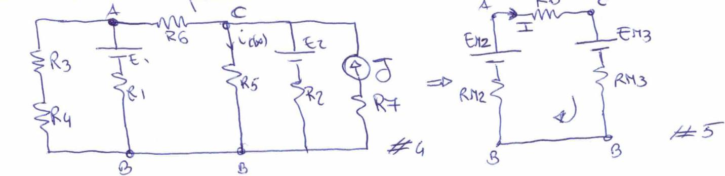
$$E_{H2} = \frac{\frac{E_1}{R_1}}{\frac{1}{R_1} + \frac{1}{R_3 + R_4}}$$
