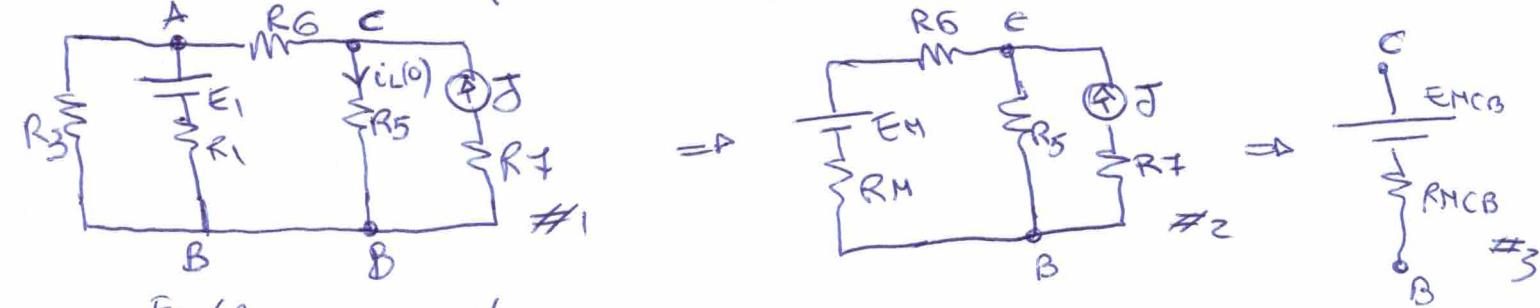
$$E_H = \frac{E_1 / R_1}{1/R_1 + 1/R_3} = 1.5 V \quad R_H = \frac{1}{\frac{1}{R_1} + \frac{1}{R_3}} = 0.95 \Omega$$
