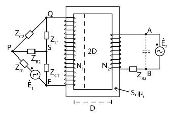
$$Z_{R_1} = R_1; \quad Z_{R_2} = R_2; \quad Z_{R_3} = R_3; \quad Z_{C_1} = \frac{1}{i\omega C_1}; \quad Z_{C_2} = \frac{1}{i\omega C_2}; \quad Z_{L_1} = i\omega L_1;$$
