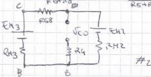
$$E_{H3} = \frac{E_{H1}}{\frac{1}{(R_{H1} + R_{57})} + \frac{1}{R_3}} = 1.6V$$
