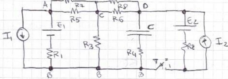
$E_1 = 8V$     $E_2 = 7V$     $I_1 = 1A$     $I_2 = 1.5A$     $R_1 = R_3 = R_5 = R_7 = 4\Omega$
