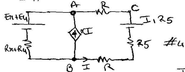
$$\begin{cases} V_{AB} = (E_M + E_A) + (R_H + R_u)(\alpha + 1)I \\ V_{AB} = I_1 R_5 - I(R_5 + R_u) \end{cases}$$
