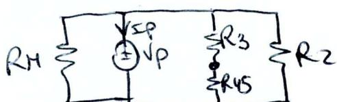
$$R_{VL} = \left[ (R_3 + R_{45}) \parallel R_2 \right] \parallel R_H$$
