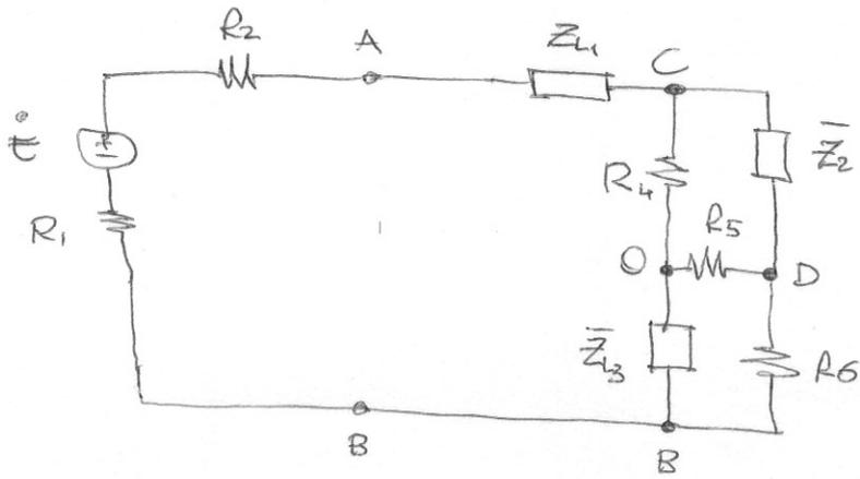
$$\begin{aligned} \dot{E} &= k_M \\ \bar{Z}_1 &= j\omega L_1 \\ \bar{Z}_2 &= R_3 + j\omega L_2 \\ \bar{Z}_3 &= j\omega L_3 \end{aligned}$$
