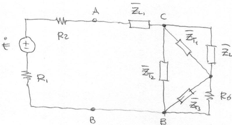
$$\begin{aligned} \bar{Z} &= \frac{1}{\frac{1}{R_4} + \frac{1}{R_5} + \frac{1}{\bar{Z}_3}} \\ \bar{Z}_{T1} &= \frac{R_4 R_5}{\bar{Z}} \\ \bar{Z}_{T2} &= \frac{R_4 \bar{Z}_3}{\bar{Z}} \\ \bar{Z}_{T3} &= \frac{R_5 \bar{Z}_3}{\bar{Z}} \end{aligned}$$
