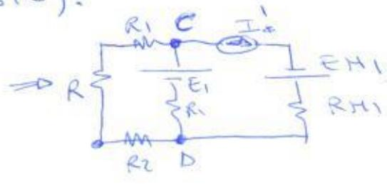
$$E_{TH1} = \frac{\frac{E_2}{R_2} + \frac{E_3}{R_3}}{\frac{1}{R_2} + \frac{1}{R_3} + \frac{1}{R}}$$
