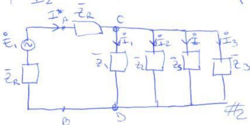
$$\begin{aligned} \bar{Z}_R &= 3\Omega \\ \bar{Z}_S &= \alpha + R_2 = 4\Omega \\ \bar{Z}_3 &= j\omega L_3 \end{aligned}$$
