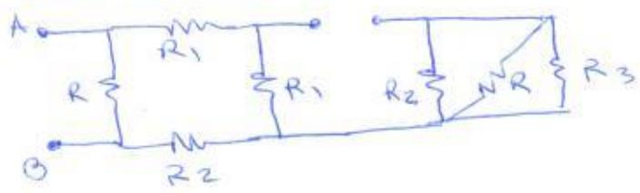
$$R_{TH} = R \parallel (R_1 + R_1 + R_2)$$
