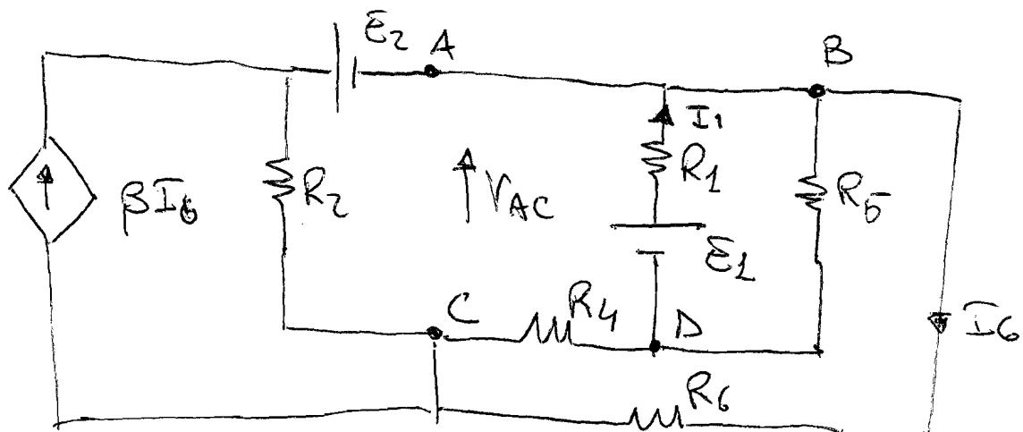
$$V_{BC} = R_6 I_6 \Rightarrow I_6 = \frac{V_{BC}}{R_6}$$
