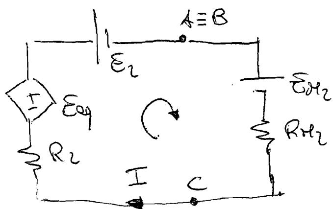
$$\left\{ \begin{array}{l} E_2 + E_{H2} - Eq + (R_2 + R_{H2}) I = 0 \\ V_{BC} = E_{H2} + R_{H2} I \end{array} \right.$$
