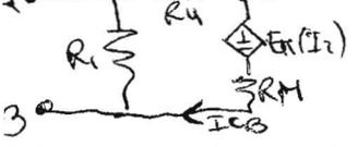
$$V_{AB}(0) = V_{AC} + V_{CB} = V_p + [E_{TH}(I_2) + I_{CB} \cdot R_{TH}] = V_p + E_{TH}(I_2) + R_{TH}(I_{AC} - I_p) = V_p + E_{TH}(I_2) + R_{TH} \left( \frac{V_p}{R_4} - I_p \right)$$
