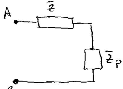
$$\begin{aligned}\bar{Z}_P &= \frac{1}{\frac{1}{\bar{Z}_C} + \frac{1}{\bar{Z}_L} + \frac{1}{\bar{Z}_R}} = \frac{\bar{Z}_C \cdot \bar{Z}_L \cdot \bar{Z}_R}{\bar{Z}_L \bar{Z}_R + \bar{Z}_C \bar{Z}_R + \bar{Z}_C \bar{Z}_L} = \\ &= \dots = \frac{\frac{L}{C} R}{\frac{L}{C} + j(\omega L R - \frac{R}{\omega C})}\end{aligned}$$
