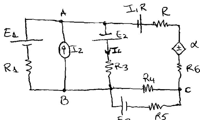
$$E_H = \frac{\frac{E_1}{R_1} + I_2 - \frac{E_2}{R_3}}{\frac{1}{R_1} + \frac{1}{R_3}}$$
