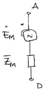
Risulta:  $\dot{V}_{AD} = \dot{E}_M = \frac{\frac{\dot{E}}{\bar{Z}_{R1}}}{\frac{1}{\bar{Z}_{R1}} + \frac{1}{\bar{Z}_{RL}} + \frac{1}{\bar{Z}_{e1} + \bar{Z}_{p3}}} = 3,83 + j 5,16 \text{ V}$
