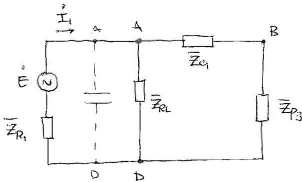
$$\bar{Z}_{p3} = \frac{(\bar{Z}_{p1} + \bar{Z}_{p2}) \cdot \bar{Z}_{R3L2}}{\bar{Z}_{p1} + \bar{Z}_{p2} + \bar{Z}_{R3L2}} = 2,77 - j 4,59 \Omega$$
