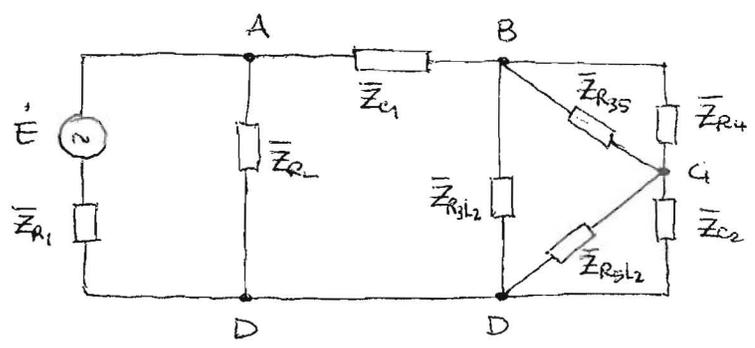
indicato con:  $\bar{Z}_p = \frac{1}{\frac{1}{\bar{Z}_{R3}} + \frac{1}{\bar{Z}_{R5}} + \frac{1}{\bar{Z}_{L2}}} = 1,87 + j0,06 \Omega$
