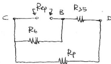
$$R_p = \frac{R_4 R_5}{R_4 + R_5}$$
